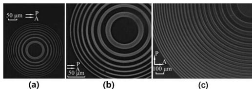
Fig. 2. Optical microphotograph of the designed LCFZL. (a) LCFZL (lens I) with  $f = 3.2$  mm under parallel polarizers, (b) the enlarged image of the lens I shown in (a), and (c) LCFZL (lens II) with  $f = 50$  mm under crossed polarizers.
