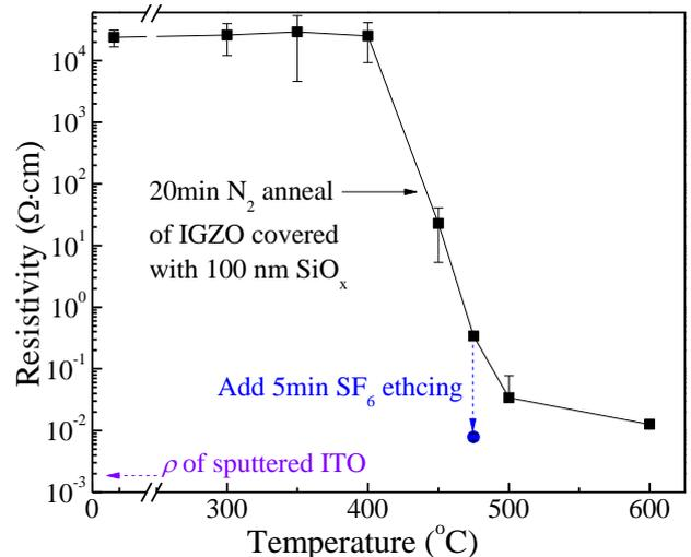
Figure 5. The temperature-dependence of the  $\rho$  of IGZO/ $SiO_x$  sample subjected to 20-minute anneals in  $N_2$ .
