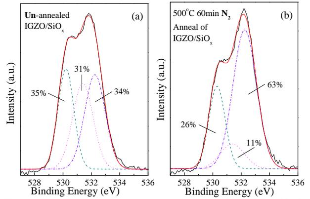
Figure 4. The XPS spectra of O 1s for IGZO/ $SiO_x$  sample (a) un-annealed or (b) subjected to 500 °C 60-minute anneal in  $N_2$ .
