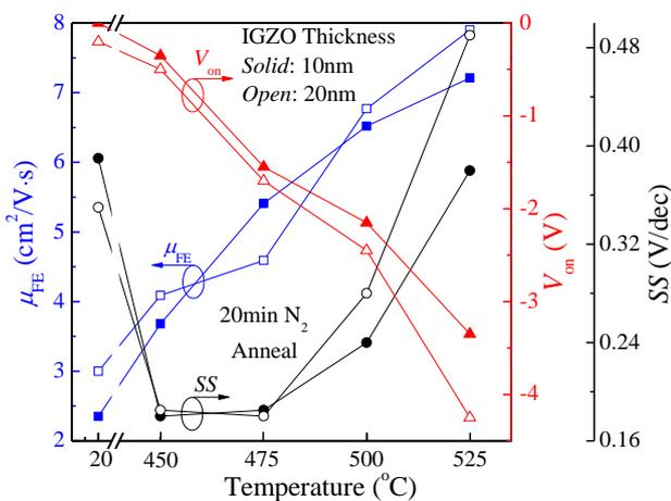
Figure 3. The temperature-dependence of  $\mu_{FE}$ ,  $V_{on}$  and SS for the annealed TFTs.
