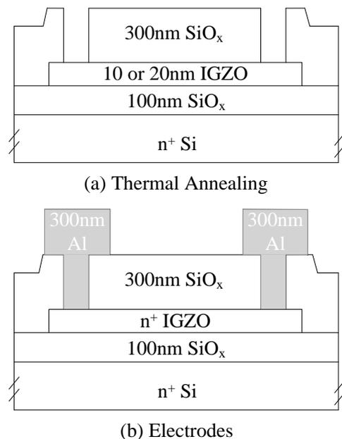
Figure 1. The schematic cross-section of an IGZO TFT during (a) thermal annealing and (b) electrode patterning.
