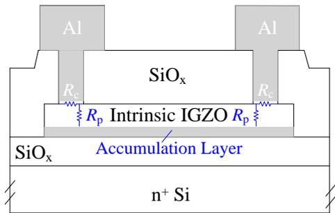
Figure 6. The schematic cross-section of an IGZO TFT, indicating the presence of  $R_p$  and  $R_c$ .
