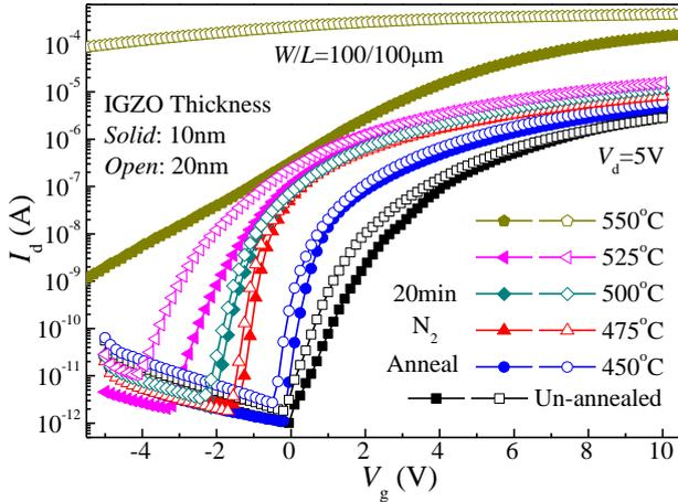
Figure 2. The transfer characteristics of IGZO TFTs subjected to a series of 20-minute isochronal anneals in  $N_2$  at different temperatures.
