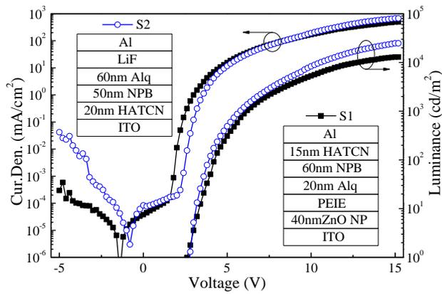
Figure 8. (a) Current density-voltage and (b) luminance-voltage characteristics of the proposed inverted OLED compared with those of conventional OLED.
