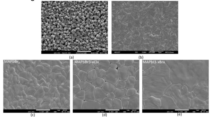
Figure 4. Sample SEM images of (a) solution processed MAPbI<sub>3</sub>, (b) css processed MAPbI<sub>3</sub>, (c) css processed MAPbBr<sub>3</sub>, (d) css processed MAPbBr<sub>3</sub>-xClx, (e) css processed MAPbI<sub>3</sub>-xBrx.
