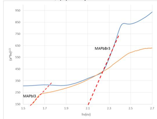
Figure 5. Tauc plot of MAPbI<sub>3</sub> and MAPbBr<sub>3</sub>
