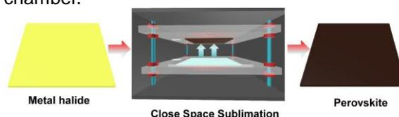
Figure 1. Schematic of close space sublimation of perovskites
