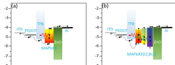
Figure 6. perovskite light emitting diode structure of (a) single layer, (b) multilayers.
