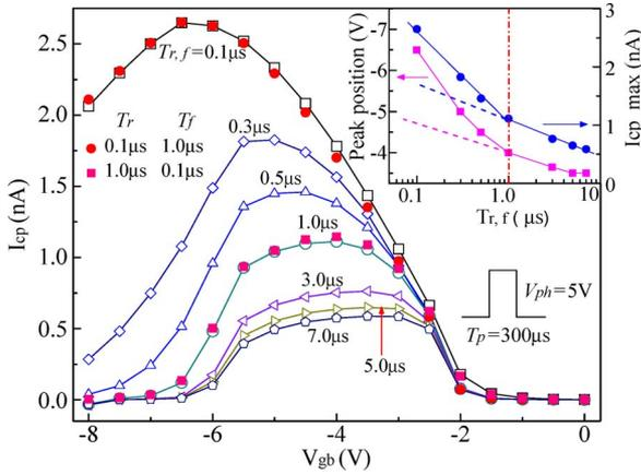
Fig. 2. Elliot curves for HT devices using square pulses with different  $T_r$ 's and  $T_f$ 's. The inset shows the peak position and  $I_{cp\_max}$  (the  $I_{cp}$  values at the corresponding peak positions) that are dependent on  $T_{r,f}$ . At  $T_r \gg 1 \mu s$ ,  $I_{geo}$  is minimized, and improved CP curves are obtained.
