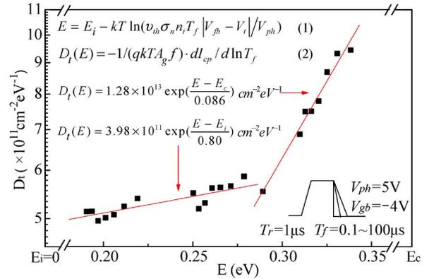
Fig. 4. Typical dual exponential  $D_t(E)$  distribution between the midgap ( $E_i$ ) and the conduction band ( $E_c$ ) for HT devices extracted with (1) and (2) using optimized square pulses.
