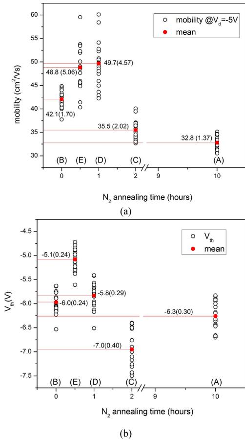
Fig. 3. The distributions of (a) field-effect mobility and (b) threshold voltage for sample A, B, C, D, and E. The mean and standard deviation (in the brackets) are labeled on the figures.
