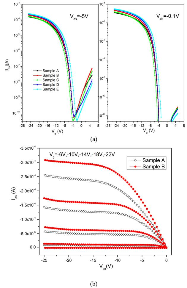
Fig. 2. (a) Transfer and (b) output characteristics of the poly-Si MIC TFTs.
