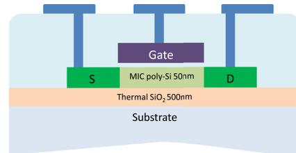
Fig. 1. Cross-sectional schematic of the poly-Si TFTs with self-aligned structure.
