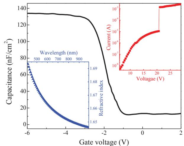
**Fig.3: Capacitance density of Si/Al<sub>2</sub>O<sub>3</sub>/Al capacitor with area of 50μm×50μm, measured at the frequency of 1kHz. The upper inset is the breakdown voltage test and the lower inset the *n* dependent on wavelength determined by ellipsometer.**
