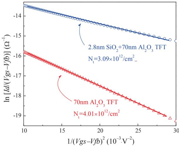
**Fig.6:**  $\ln[I_d/(V_{gs}-V_{fb})]$  versus  $1/(V_{gs}-V_{fb})^2$  curves at  $V_{ds}=-0.1V$  for LTPS TFTs using  $Al_2O_3$  gate dielectric with/without buffer thermal oxide.
