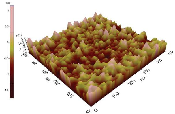
**Fig.2: AFM image of the 70nm Al<sub>2</sub>O<sub>3</sub> film sputtered on bare Si wafer.**
