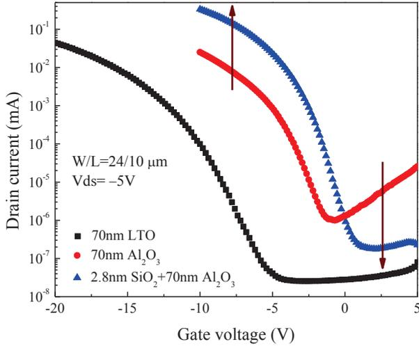
**Fig.4:** The transfer curves of LTPS TFTs with different gate dielectrics, measured at  $V_{ds}=-5V$ .
