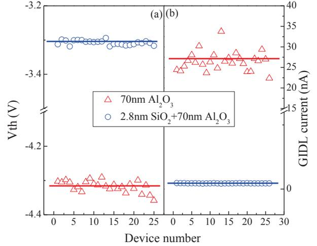
**Fig.7:** (a)  $V_{th}$  and (b) GIDL current variations for 25 TFTs with  $Al_2O_3$  gate dielectric and 25 TFTs with thermal oxide buffered  $Al_2O_3$  gate dielectric.
