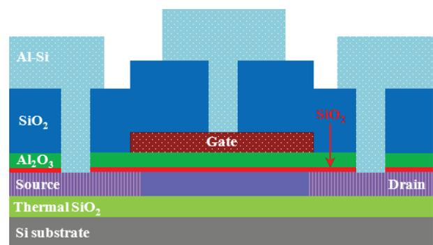
**Fig.1: The cross-sectional schematic of poly-Si SPC TFTs using thermal oxide buffered  $Al_2O_3$  as gate dielectric.**
